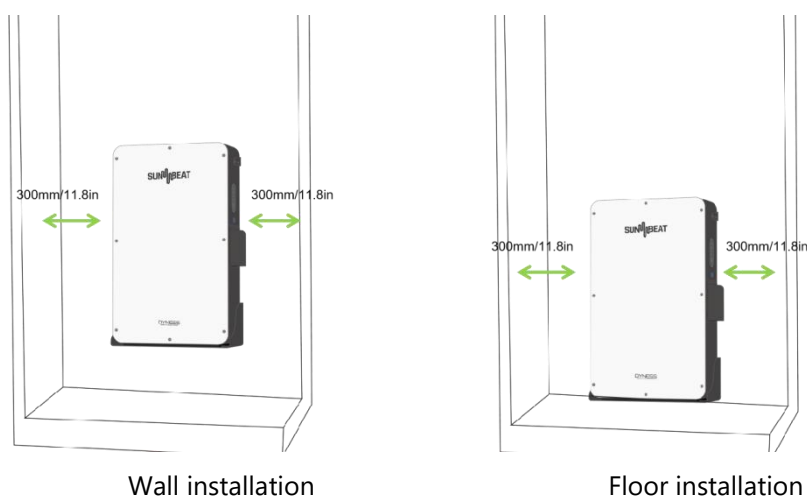
Figure 3-3 Mounting Space Requirements
